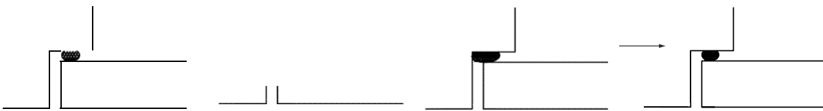
Figure A.34 a) - Dimension of draught/smoke seals (Euroclass A1) - leaf or frame fitted - Increase
